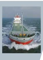
in terms of length, width or draft due to specific channels or locks. Take the EasyMax, for example: here we deliberately opted for a maximum draft of 8.60 metres, because this also allows the ship to navigate the Saint Lawrence and the Great Lakes on the other side of the Atlantic."
