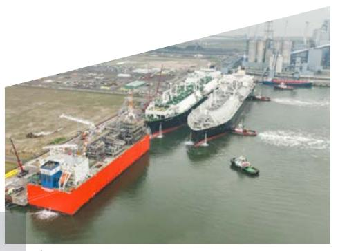
The incoming tankers transporting LNG moor ship-to-ship against the Golar Igloo to unload. From there, the gas can be transferred to the Eemshaven LNG.
